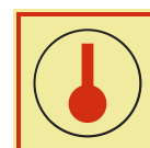
92318 H Spaces monitored by heat detector(s)
