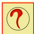
92315 H Space or group of spaces monitored by smoke detector(s)
