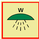
92215-W H space or group of spaces protected by fire- extinguishing system
