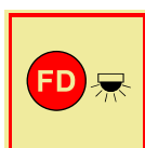
92206 H Space protected by automatic fire alarm
