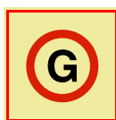
92300 H Emergency source of electrical power (generator)
